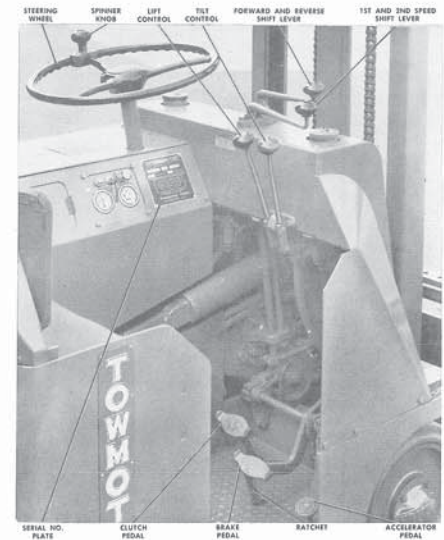
Fig. 1. Driving and Lifting Controls
