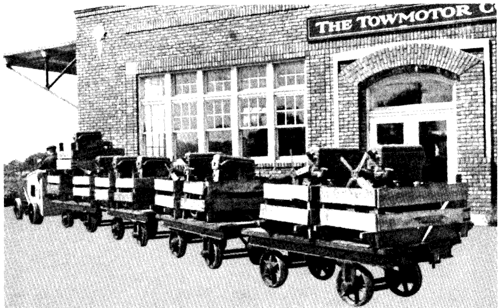
Model A Towmotor pulling trailers loaded with motors into the first plant occupied by The Towmotor Co. In this plant, located on Bliss Road, Euclid, Ohio, the pioneering, development and early production of straight gasoline-powered Towmotor industrial tractors first got under way.
